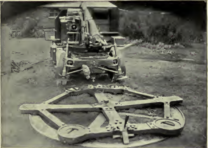
No. 2.—The turntable in position, ready to receive the gun.
