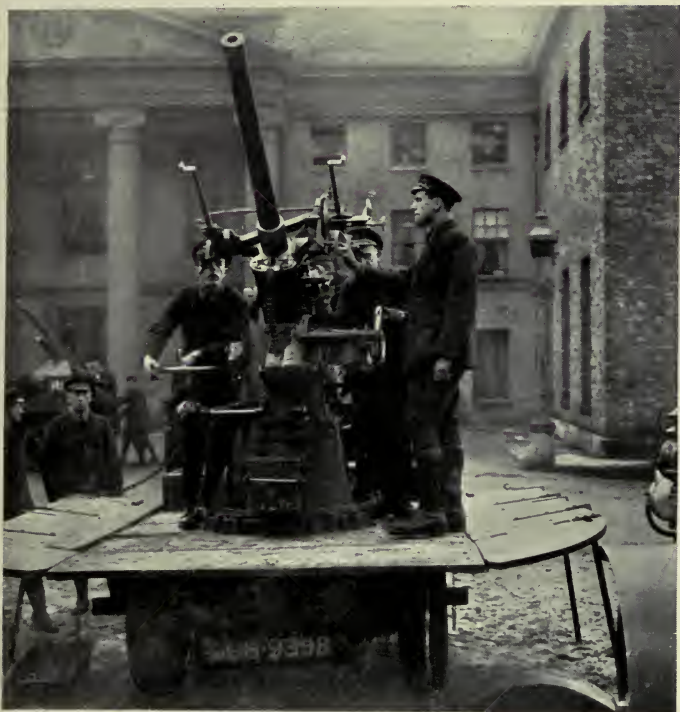
No. 1.—3-pounder Vickers' Q.F. high-velocity gun on high-angle anti-aircraft mounting and Lancia chassis.
